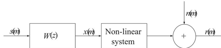
Figure 1. Non-linear channel used in the experiments.
