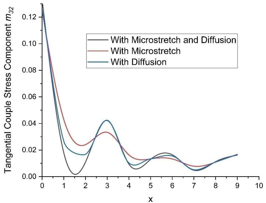
Figure 5. The variation in the tangential couple stress component  $m_{32}$  with respect to distance  $x$ .
