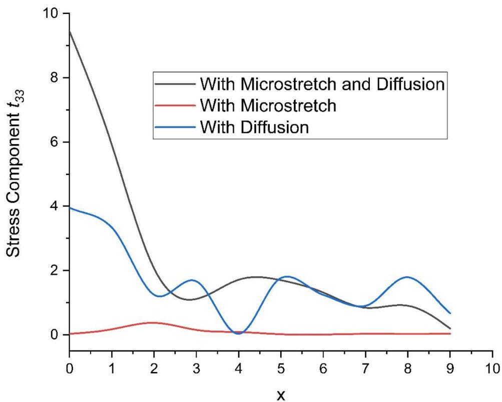
Figure 3. The variation in the stress component  $t_{33}$  with respect to distance  $x$ .
