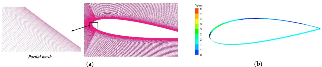
**Figure 2.** (a) Computational domain mesh diagram of the NACA0015 hydrofoil; (b) Wall surface  $Y_{plus}$  diagram of the NACA0015 hydrofoil.
