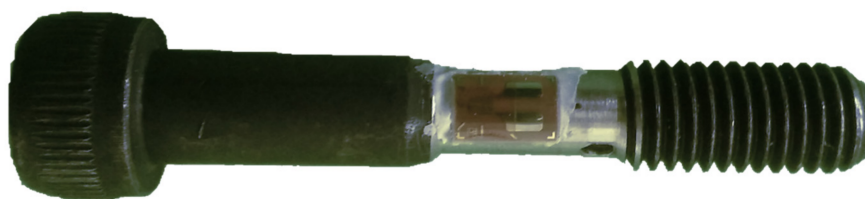
Figure 5. Bolt with bonded strain gauges.
