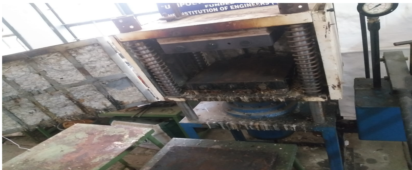
Figure 30. Composite Compression Molding.
