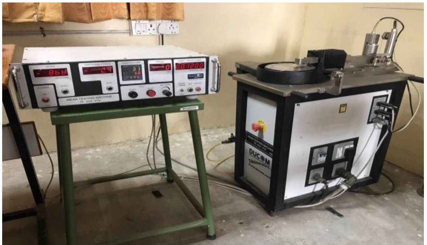
Figure 32. A typical view of another pin on disc experiment with test specimen.
