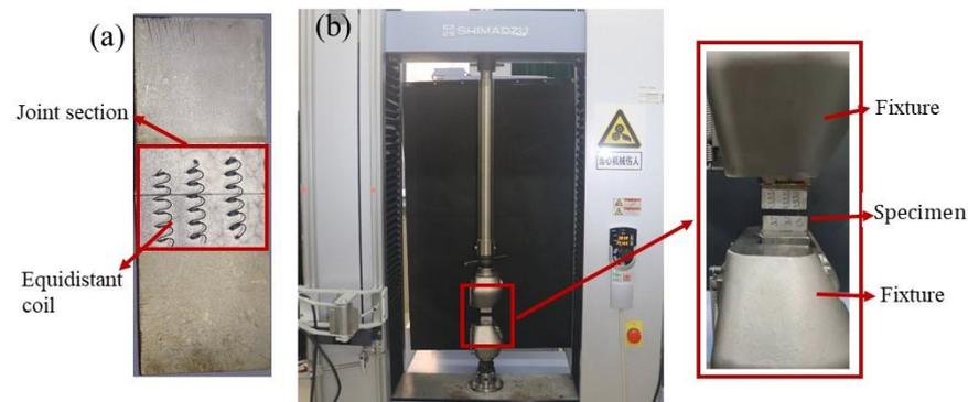
**Figure 6.** Mode-II experiment: (a) the specimen, (b) experiment setup.
