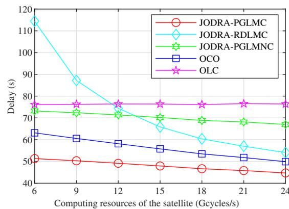
Figure 6. Delay vs. computing resources of the satellite.
