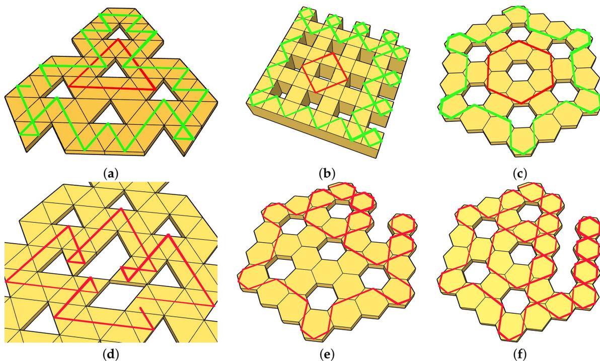
**Figure 2.** (a–c) Internal and edge modes on the photonic topological insulators assembled from triangular, quadrangular, and hexagonal glass prisms. (d–f) Edge modes.
