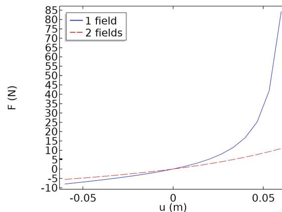
**Figure 5.** Comparison between numerically computed reaction forces for compressive-extension tests for 1-field model (blue, full line) and 2-fields model (red, dashed line). Same constitutive parameters are used for the two models.
