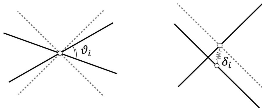
**Figure 3.** Kinematics of connective elements, hinges or pivots, depicting torsion (left) and micro-shear (right) mechanisms.
