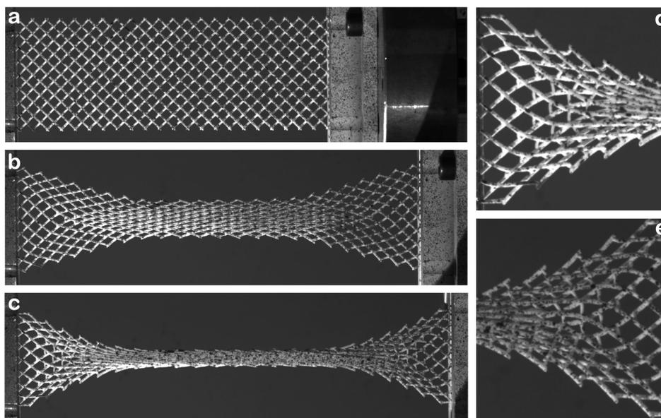
**Figure 4.** Experimental observation of micro-shear of pivots in an extension test of a 3D-printed specimen. In (a–c), three different deformation stages are shown. In (d,e), the extremities of the sample in (c) are magnified for showing the micro-shear of pivots. The author acknowledges Prof. F. Hild and Mr. X. Pinelli of Paris-Saclay University for their help in performing experimental measures.
