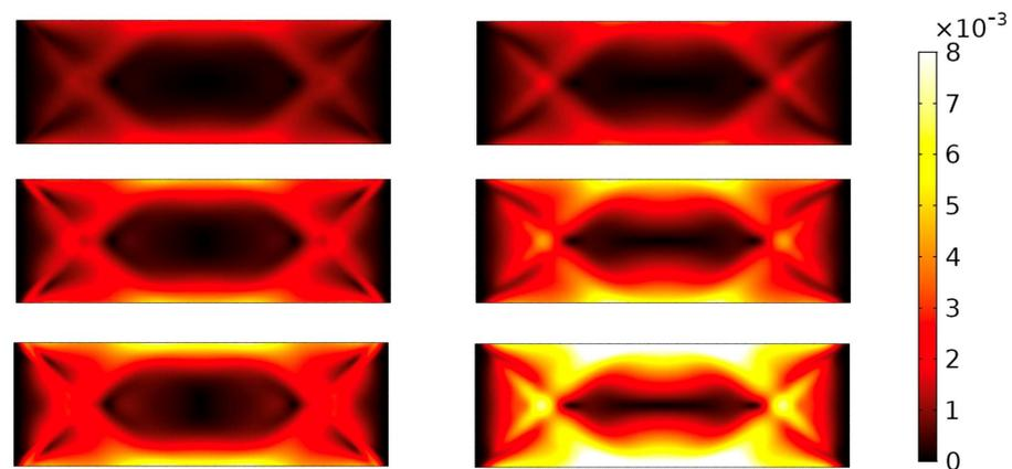
**Figure 8.** Plot of relative displacements of the two fiber families. The absolute value of displacement is represented in the color scale, expressed in m. The plots are reported for different values of prescribed displacement:  $-20$  mm,  $-40$  mm and  $-60$  mm in compression (left);  $20$  mm,  $40$  mm and  $60$  mm in extension (right).
