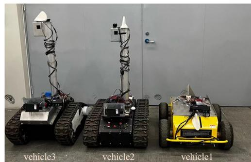
**Figure 10.** Three micro-vehicles for the experiment.
