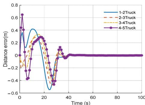
(c) Distance tracking error with the proposed method
