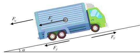
**Figure 2.** Force analysis of a vehicle on the ramp.
