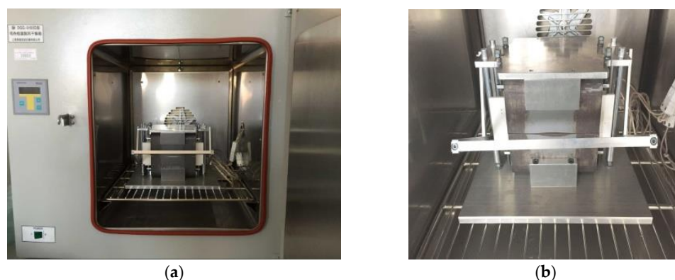
Figure 1. Temperature effect measuring instrument for magnetic characteristics. (a) thermostat (b) magnetic property measuring instrument SST.
