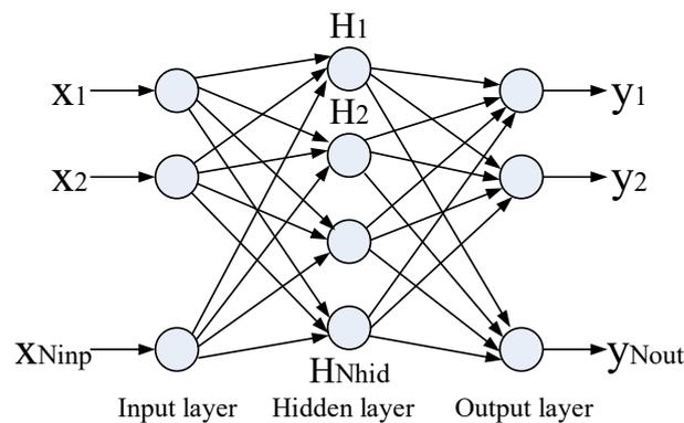
Figure 7. The basic architecture of the neural network.
