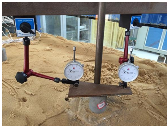
Figure 8. Layout showing the dial indicators placed on top of the pile.
