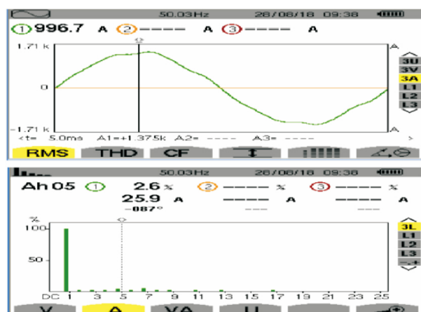
Figure 11. U-phase current of the harmonic source and its harmonic spectrum with DTPF.
