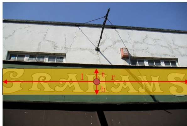
Figure 3. The proposed method predicts a 4D vector ( l , t , r , b ), where l , t , r , b are the distances from the location to the four sides of the bounding box.
