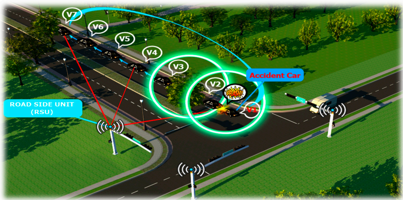
Figure 1. Single-lane, high-speed road traffic scenario: using vehicle-to-vehicle (V2V) and vehicle-to-road (V2R) or road-to-vehicle (R2V) communication protocols for road and public efficiency and safety.
