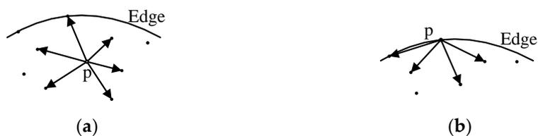
Figure 3. The edge distribution characteristics of the point cloud. (a) Neighborhood distribution of non-edge points; (b) Neighborhood distribution of edge points.
