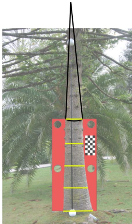
**Figure 10.** Tree segmentation method. The yellow lines represent four tree base sections approximated as truncated cones. The black lines represent the remaining tree stem, approximated as a cone (not to scale in the image).
