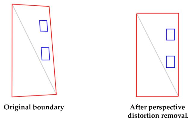
**Figure 4.** Homographic transformation to remove the perspective distortion.
