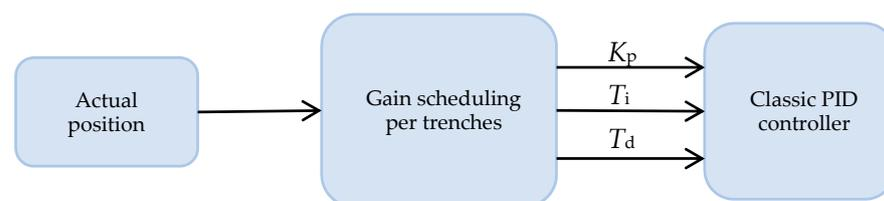
**Figure 4.** Scheme of variable PID control strategy.
