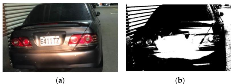
**Figure 2.** (a) A license plate captured in a bright environment, (b) the binary image generated by Otsu, where the license plate disappears.
