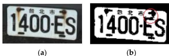
**Figure 3.** (a) A license plate on which two screws get rusty, (b) the binary image generated by Otsu, where rusty screws adhere to the Character “E.”
