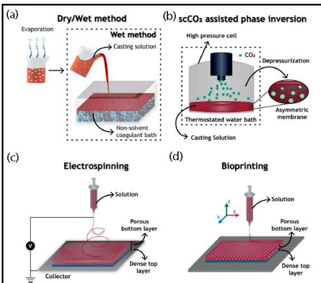
**Figure 2.** Four main methodologies for the production of asymmetric membranes: (a) dry/wet, (b)  $scCO_2$ -assisted phase inversion, (c) electrospinning, and (d) bioprinting [57].
