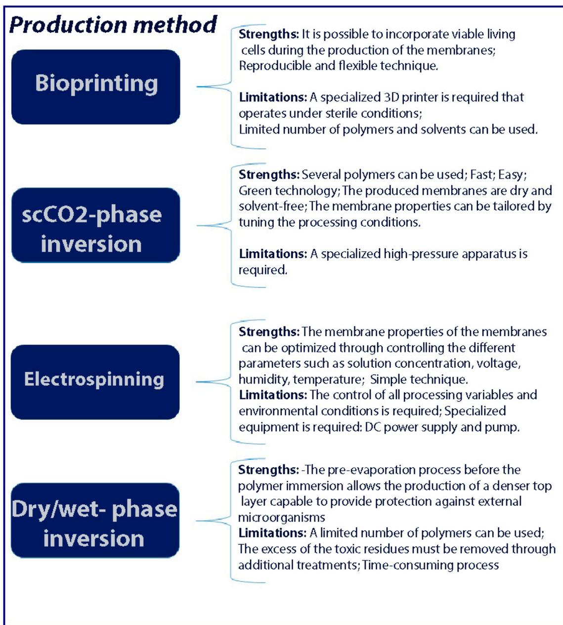
**Figure 3.** A summary of strengths and limitations of asymmetric membranes production methods.
