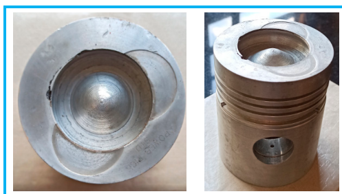
Figure 6. Top and side views of the Toroidal combustion chamber.
