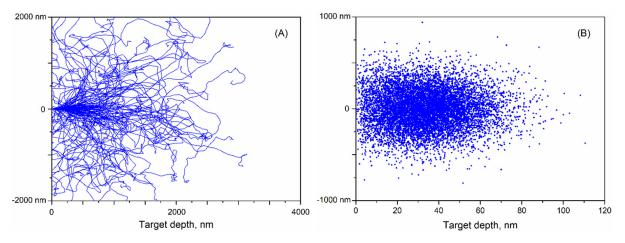
Figure 2. (A) Modeling the path for electrons of 30 keV and (B) protons of 3 keV in zinc oxide.
