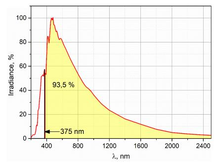
**Figure 10.** Solar radiation spectrum: 93.5% of quanta has an energy lower than the zinc oxide band gap (375 nm).
