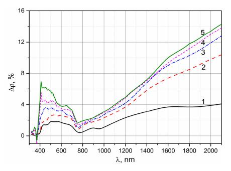
**Figure 7.**  $\Delta \rho_{\lambda}$  Spectra after irradiation of a TRSO-2M coating with 30 keV electrons, fluence values =  $0.6 \cdot 10^{15}$  (1),  $2 \times 10^{15}$  (2),  $4 \times 10^{15}$  (3),  $6 \times 10^{15}$  (4), and  $1 \times 10^{16}$  (5) cm<sup>-2</sup>.
