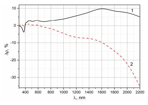
**Figure 9.**  $\Delta \rho_{\lambda}$  spectra after irradiation of ultra-high purity ZnO 14-2 pigment with 5 sre for 40 h (1) and follow-up 33-day-long storage in a residual vacuum (2).
