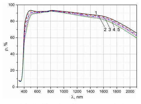
**Figure 3.**  $\rho_{\lambda}$  spectra before (1) and after irradiation of the TRSO-2M coating with a 3 keV proton fluence:  $1 \times 10^{15}$  (2),  $3 \times 10^{15}$  (3),  $6 \times 10^{15}$  (4), and  $1 \times 10^{16}$  (5).
