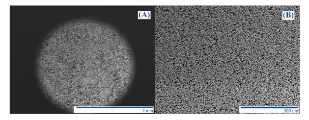
**Figure 1.** (**A**) SEM images of ZnO powder and (**B**) coating obtained by addition of 15 wt.% of potassium liquid glass.
