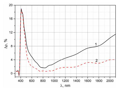
**Figure 6.**  $\Delta \rho_{\lambda}$  spectra after irradiation of the TRSO-2M coating with 3 keV protons with an energy of  $1 \cdot 10^{16}$  and after sequential irradiation with EMR, electrons (1), and follow-up EMR (2).
