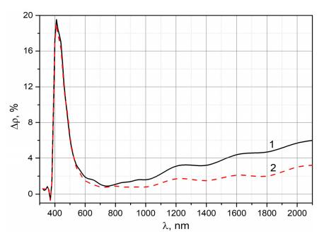
**Figure 5.**  $\Delta \rho_{\lambda}$  spectra after irradiation of the TRSO-2M coating with a 3 keV proton fluence of  $1 \times 10^{16}$  (1) and after sequential EMR (2).
