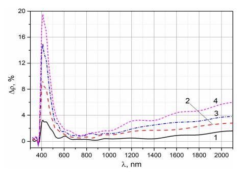
**Figure 4.**  $\Delta \rho_{\lambda}$  spectra after irradiation of the TRSO-2M coating with a 3 keV proton fluence:  $1 \times 10^{15}$  (1),  $3 \times 10^{15}$  (2),  $6 \times 10^{15}$  (3), and  $1 \times 10^{16}$  (4).
