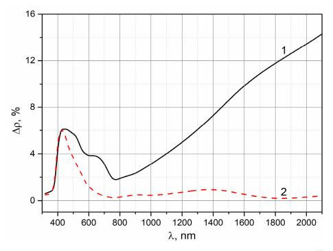
**Figure 8.**  $\Delta \rho_{\lambda}$  spectra after irradiation of a TRSO-2M coating with 30 keV electrons, F = 1 × 10<sup>16</sup> (1) and after sequential irradiation with EMR (2).
