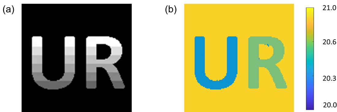
Figure 10. The 3D reconstruction results of the “U & R” target with varying reflectance: (a) the reconstructed intensity map; (b) the reconstructed depth map.
