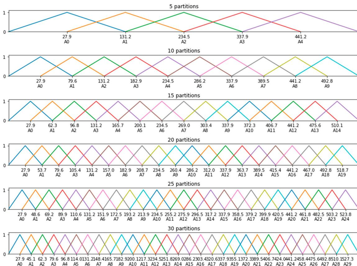
Figure 5. Partition the air pollution index data into several lengths of intervals.
