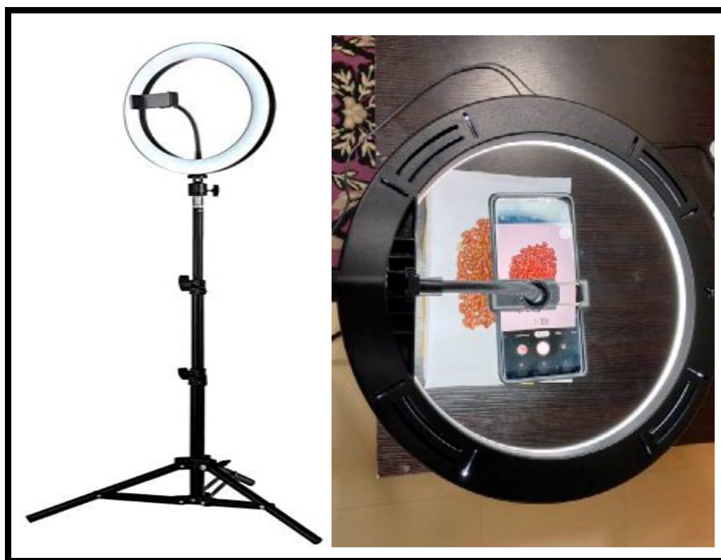
Figure 4. Setup for capturing images of seeds.
