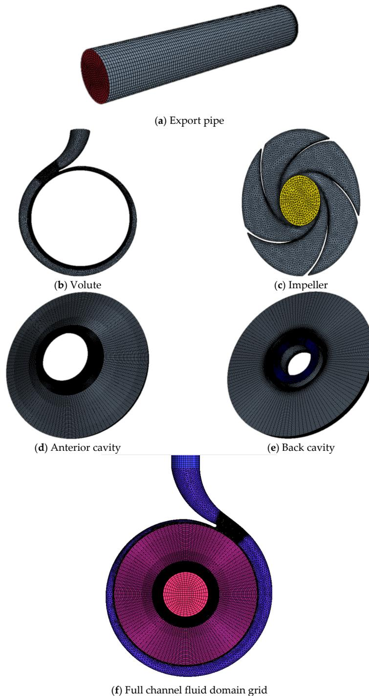
**Figure 3.** Grid of the computing model.
