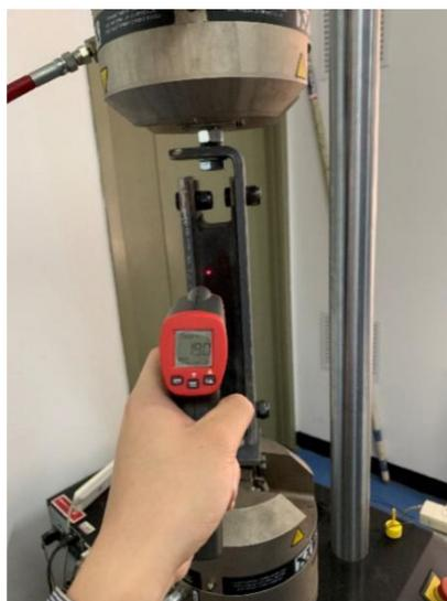
**Figure 4.** Temperature measurement of shear spring.
