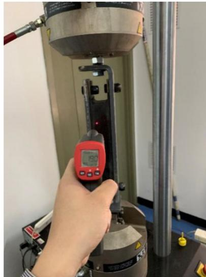
**Figure 4.** Temperature measurement of shear spring.
