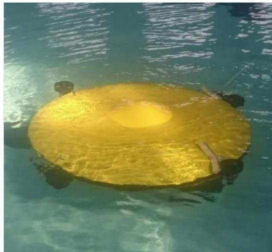
**Figure 3.** ZJU (Zhejiang University) AUH physical prototype.
