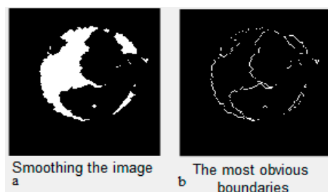
Figure 11. The outlined contours of the segmented areas of the weld nugget.
