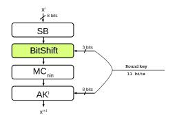
Figure 4. A BitShift key-dependent: increasing the size of the round key from 8 to 11 bits.
