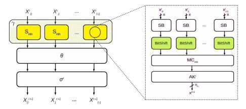
**Figure 5.** Substitution–permutation network (SPN)box: a new inner round  $\gamma$ .
