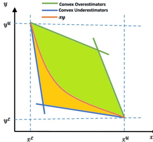
Figure 2. McCormick Envelopes: under and over estimators (reprinted).
