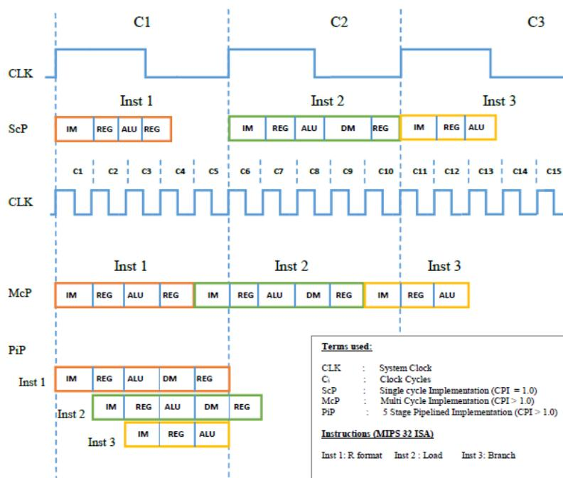
Figure 1. Timing in each processor variant.
