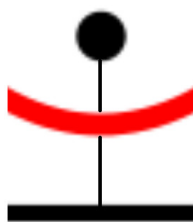
Figure 10. Profile of the vase in the form of a parabola (red curve), a directrix (bottom black straight line), a focus (top ball), and a vertical bar connecting all parts.
