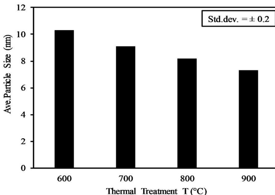
Figure 11. Effect of the CNT thermal treatment on cobalt particle size prepared at pH 14.
