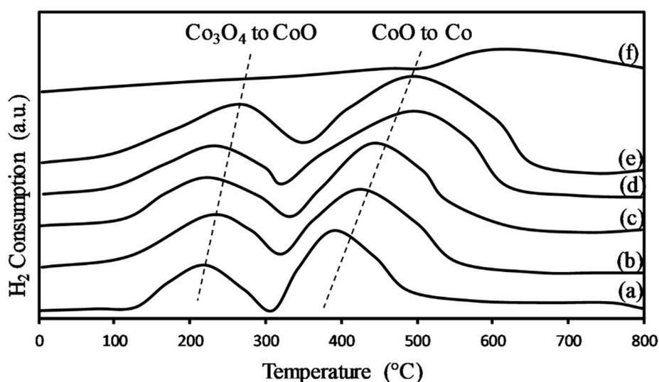
**Figure 7.** TPR-H<sub>2</sub> profile of (a) Co/CNT.5A.25, (b) Co/CNT.5A.110, (c) Co/CNT.10A.110, (d) Co/CNT.15A.110 (e) Co/CNT.20A.110, and (f) as-received CNT.
