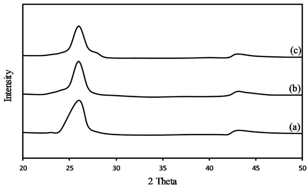
Figure 5. XRD patterns of (a) as-received CNT, (b) CNT.A.25, and (c) CNT.A.110.
