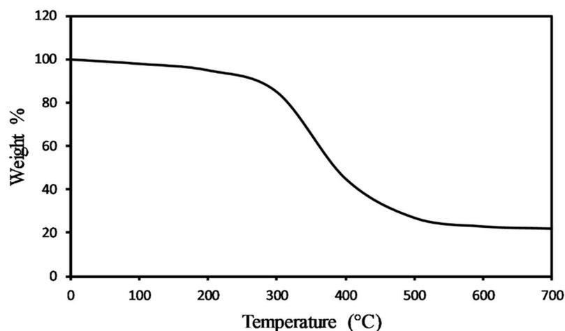
Figure 9. Thermo-gravimetric analysis of CNT.A.900 under argon flow.
