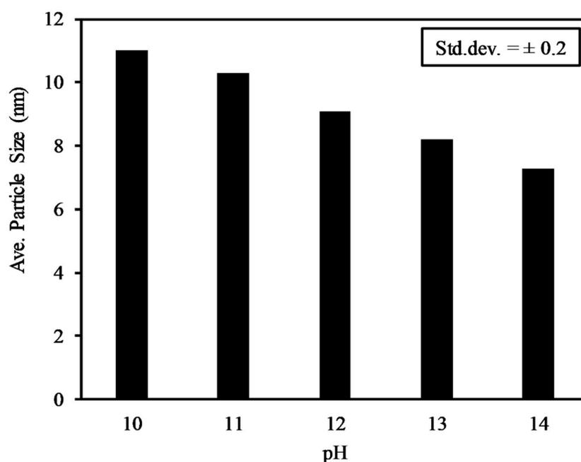
Figure 10. Effect of pH on the cobalt average particle size using CNT.A.900.
