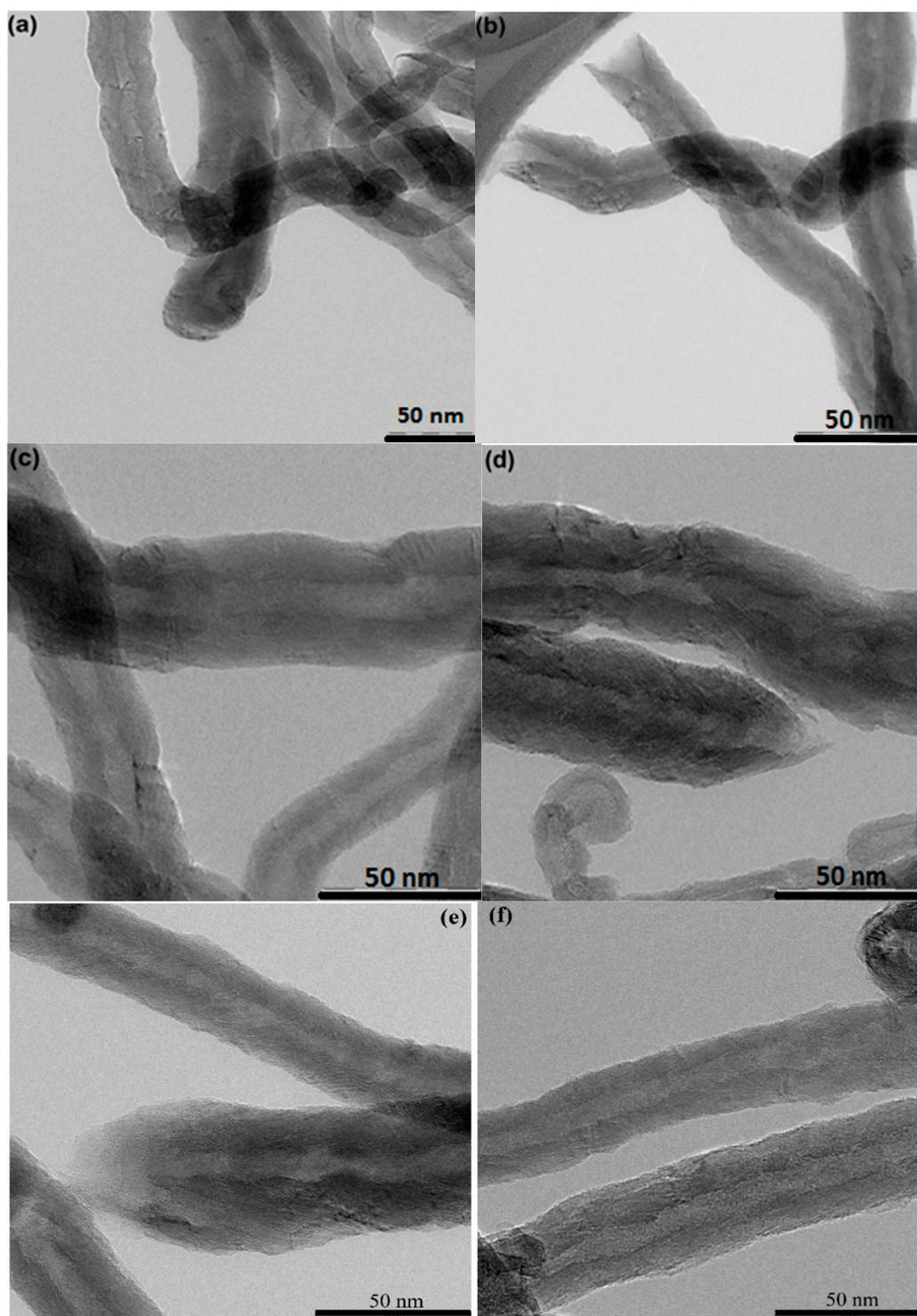
**Figure 2.** TEM images of (a) as-received CNT, (b) CNT.5A.25, (c) CNT.5A.110, (d) CNT.10A.110, (e) CNT.15A.110, and (f) CNT.20A.110.
