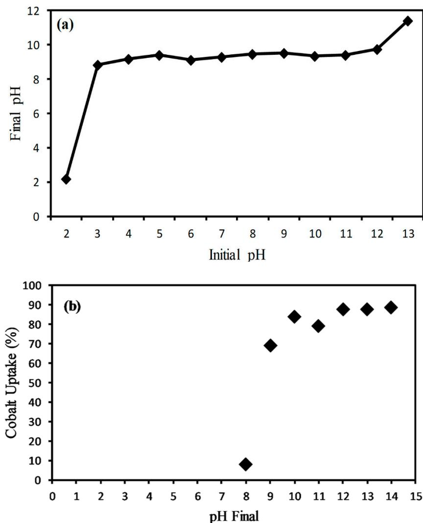
**Figure 1.** Determination of (a) point of zero charges (PZC) of the carbon nanotubes (CNT) support, and (b) Co uptake versus pH analyzed by atomic absorption spectrophotometry (AAS).
