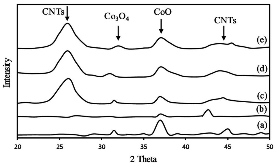
Figure 6. XRD patterns of (a)  $\text{Co}_3\text{O}_4$  standard, (b) Co/as-received CNT, (c) Co/CNT.15A.25, (d) Co/CNT.15A.110, and (e) Co/CNT.20A.110.
