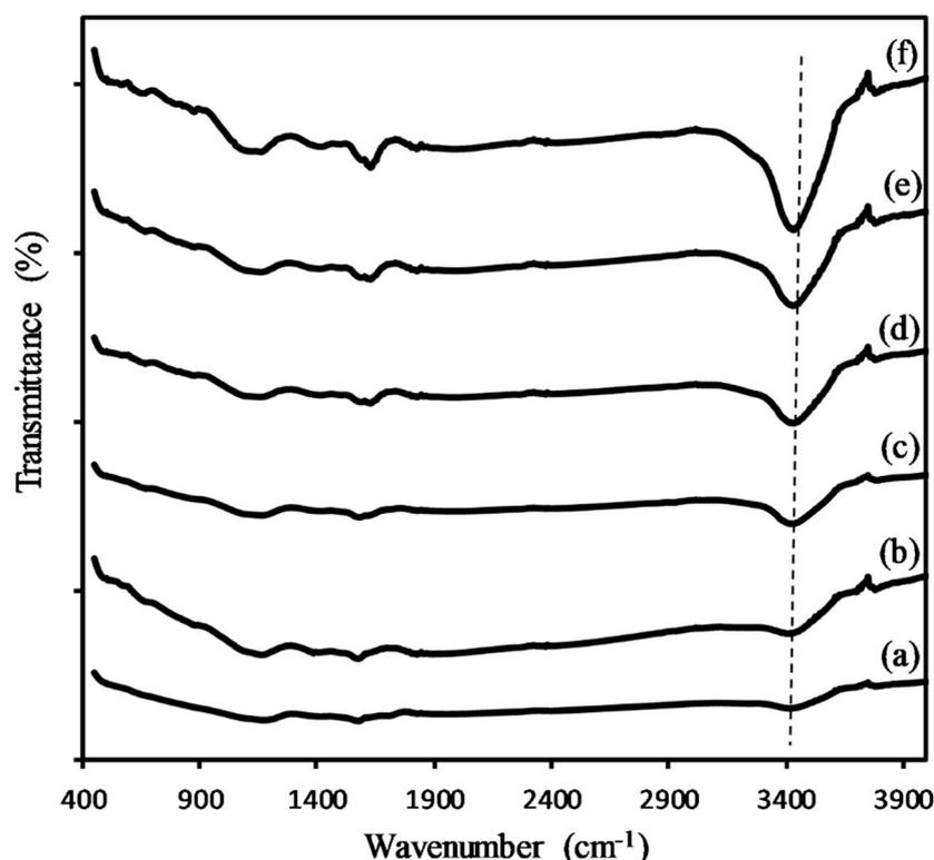
**Figure 3.** FTIR spectra of (a) as-received CNT, (b) CNT.5A.25, (c) CNT.5A.110, (d) CNT.10A.110, (e) CNT.15A.110, and (f) CNT.20A.110.
