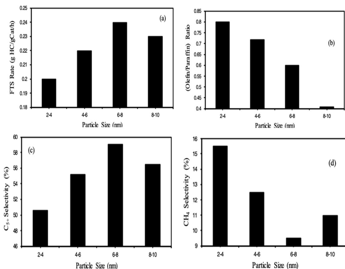
**Figure 12.** Influence of cobalt particles size on (a) FTS rate (b) olefin to paraffin ratio, (c)  $C_{5+}$  selectivity, and (d)  $CH_4$  selectivity.
