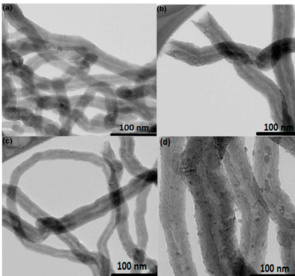
**Figure 8.** TEM images of (a) as-received CNT (b) CNT.A (c) CNT.A.900, and (d) Co/CNT.A.T900.
