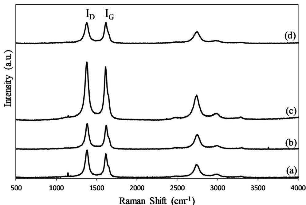
**Figure 4.** Raman spectra of (a) CNT.10A.110, (b) CNT.5A.25, (c) CNT.5A.110, and (d) as-received CNT.
