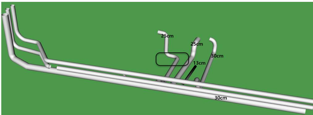
Figure 10. Predefined CAD model 2 with L joint to reduce pipe complexity.
