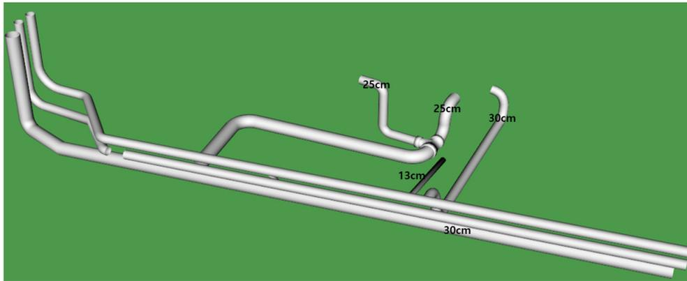
Figure 9. Predefined CAD model 1 with T joint to increase efficiency.
