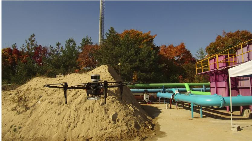
**Figure 4.** Velodyne Puck LITE sensor mounted on the chosen UAV DJI Matrice 100.
