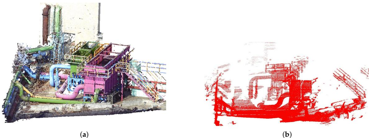
**Figure 6.** Acquired 3D PCD: (a) preprocessed, and (b) partial 3D PCD.
