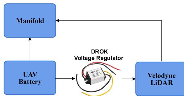
**Figure 2.** UAV and Velodyne sensor hardware integration.
