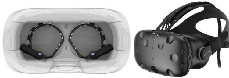
**Figure 7.** HTC Vive and Pupil eye tracker inside the HMD.
