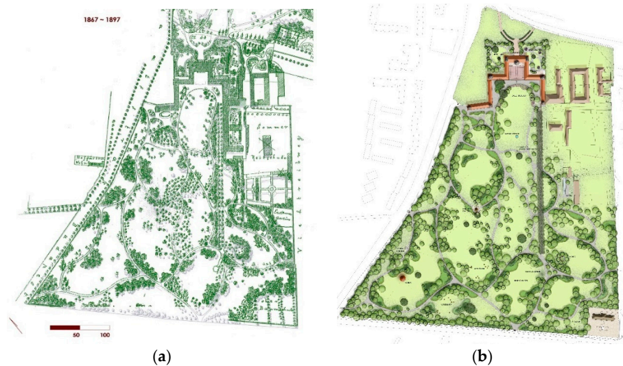
Figure 14. The restoration of visual links is related to a successful reconstruction of the spatial layout of the garden. The spatial layout is mainly determined by the vegetation, paths, and landforms. The restored path network (b) entirely corresponds to the one that existed in the Romantic landscape garden (a) in the 2nd half of the 19th century (layouts from 1867). Design by Fekete, A.; Jámbor, I.; Sárospataki, M.; Szilágyi, K.; Vajda, Sz. 2009–2010.
