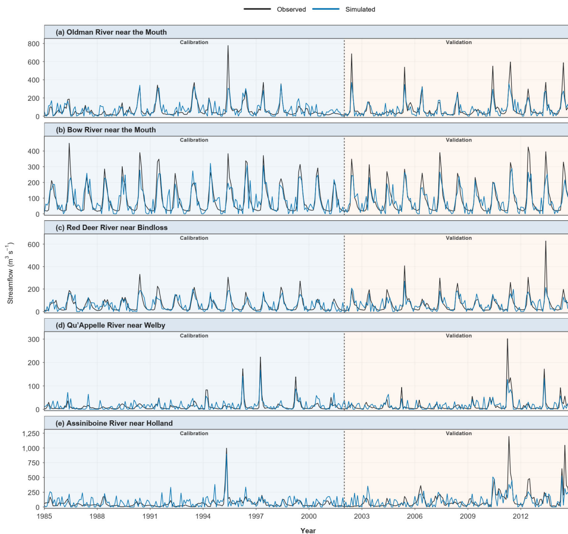
Figure 3. Monthly simulated and observed flows during the calibration period (1985–2001) and validation (2002–2014) for SWAT-M.
