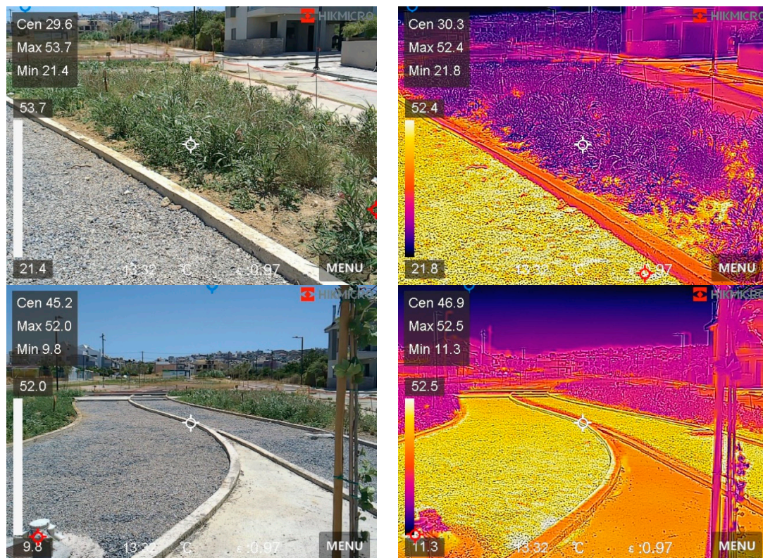
Figure A2. Indicative optical and thermal images of the urban green site in Heraklion at noon (13:30–15:30) on a warm summer day (1 August 2024), depicting the temperature ranges of various elements occupying the site. Blue and red cycles indicate the minimum and maximum temperatures, whereas white cycles show the temperature at the center of the photograph.
