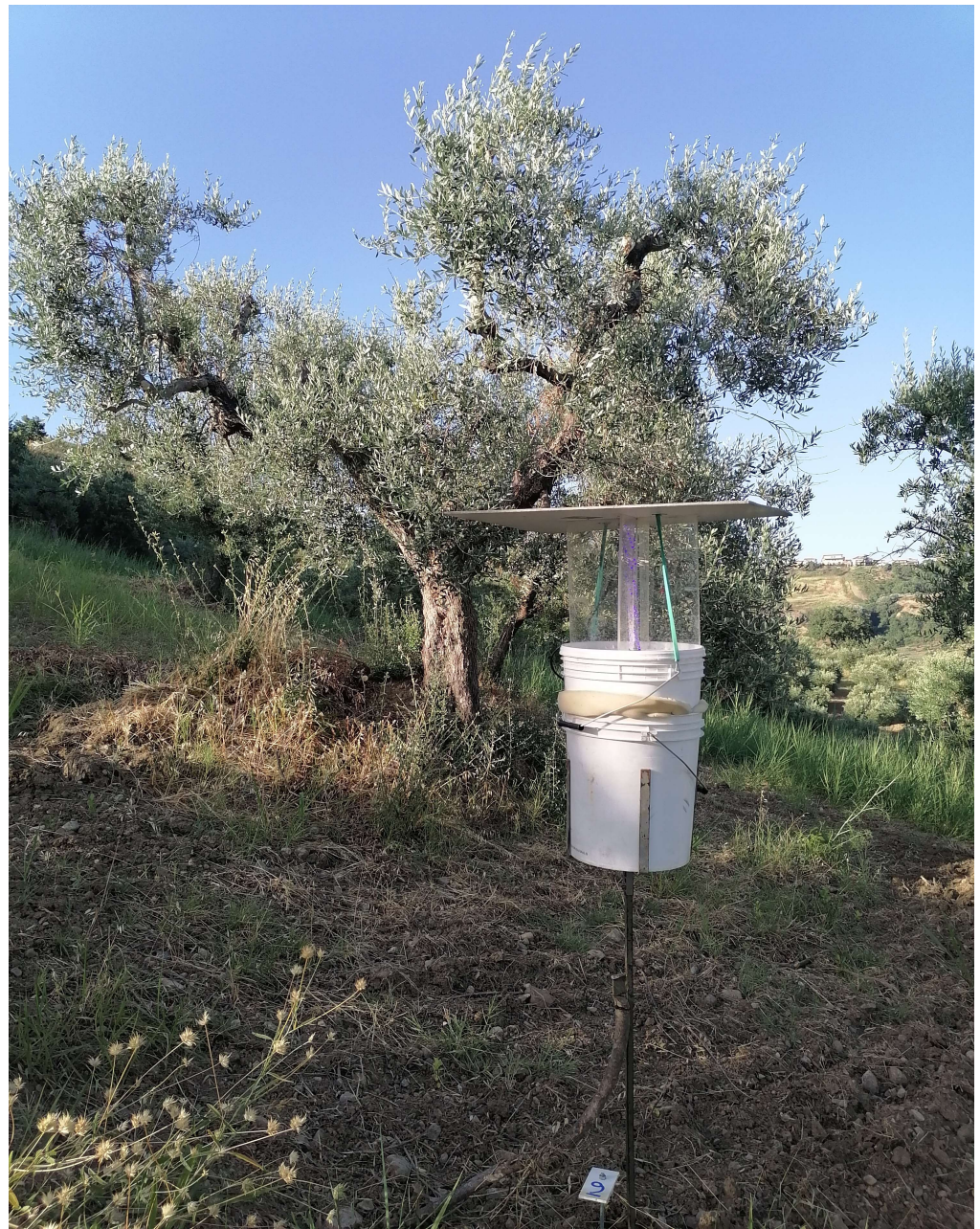
Figure 2. Used UV LED light trap positioned within the olive grove.
