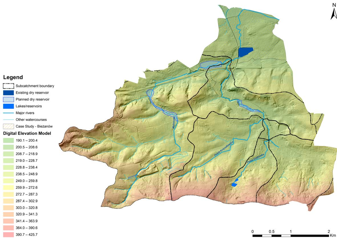
Figure 5. The digital elevation model in the Serafa River watershed.
