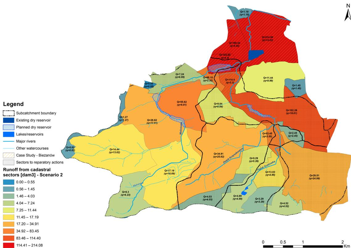
Figure 10. Accumulated and specific runoff [dam<sup>3</sup>] in cadastral sectors 100 and 101, for which reparatory measures compliant with Scenario 2 were assumed.
