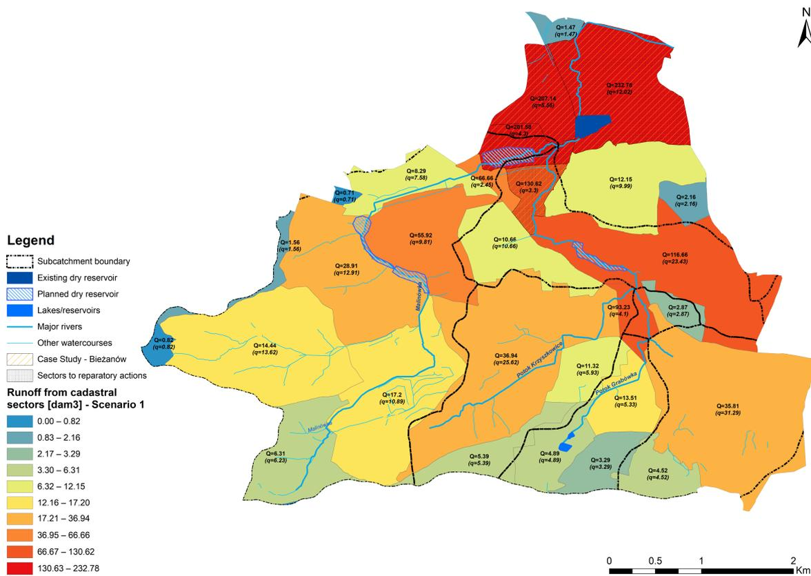
Figure 9. Accumulated ( $Q$ ) and specific ( $q$ ) runoff [dam<sup>3</sup>] in cadastral sectors 100 and 101, for which reparatory measures compliant with Scenario 1 were assumed.
