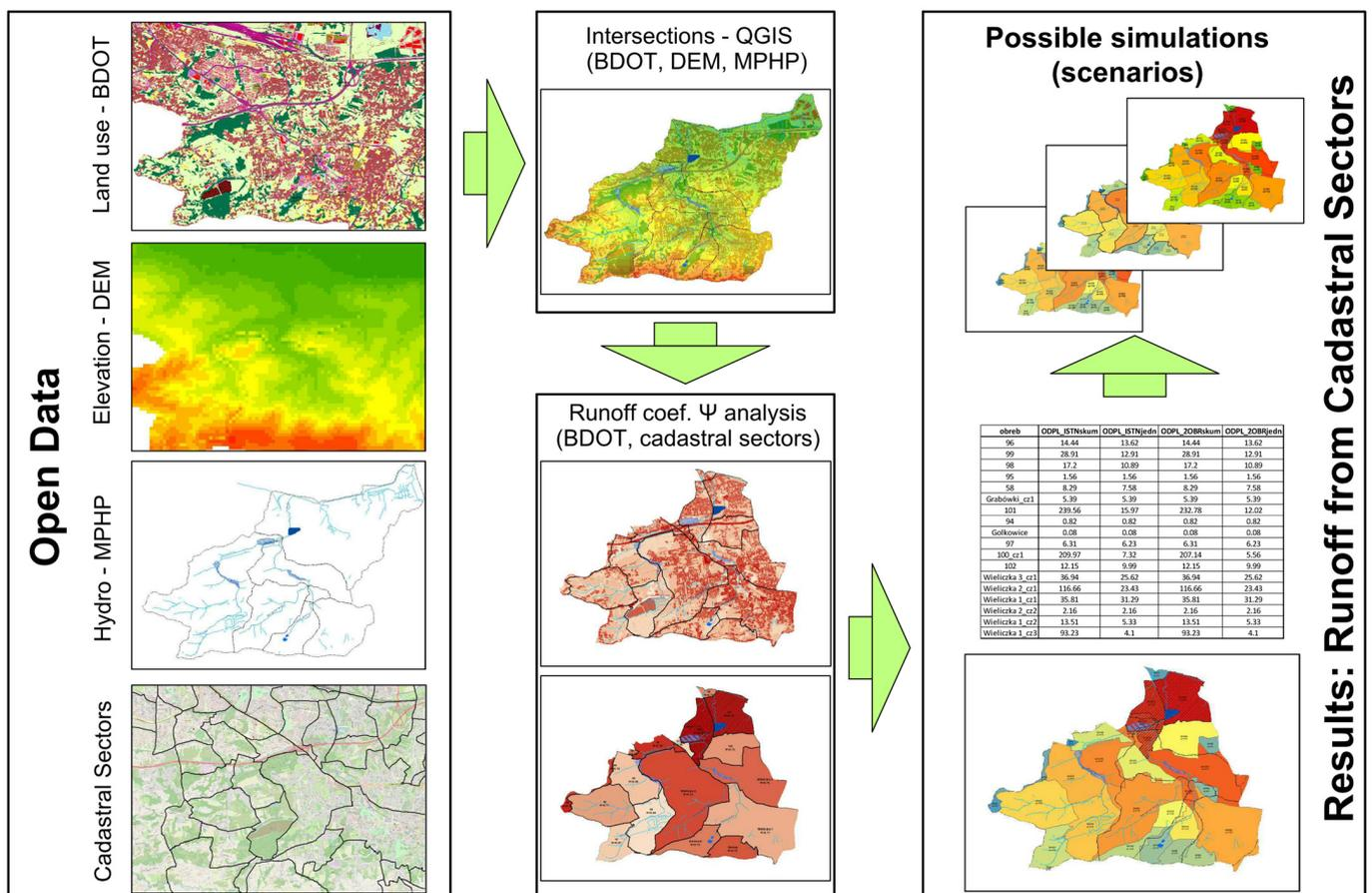
Figure 1. Flow chart showing the stages of surface runoff estimation using GIS tools.
