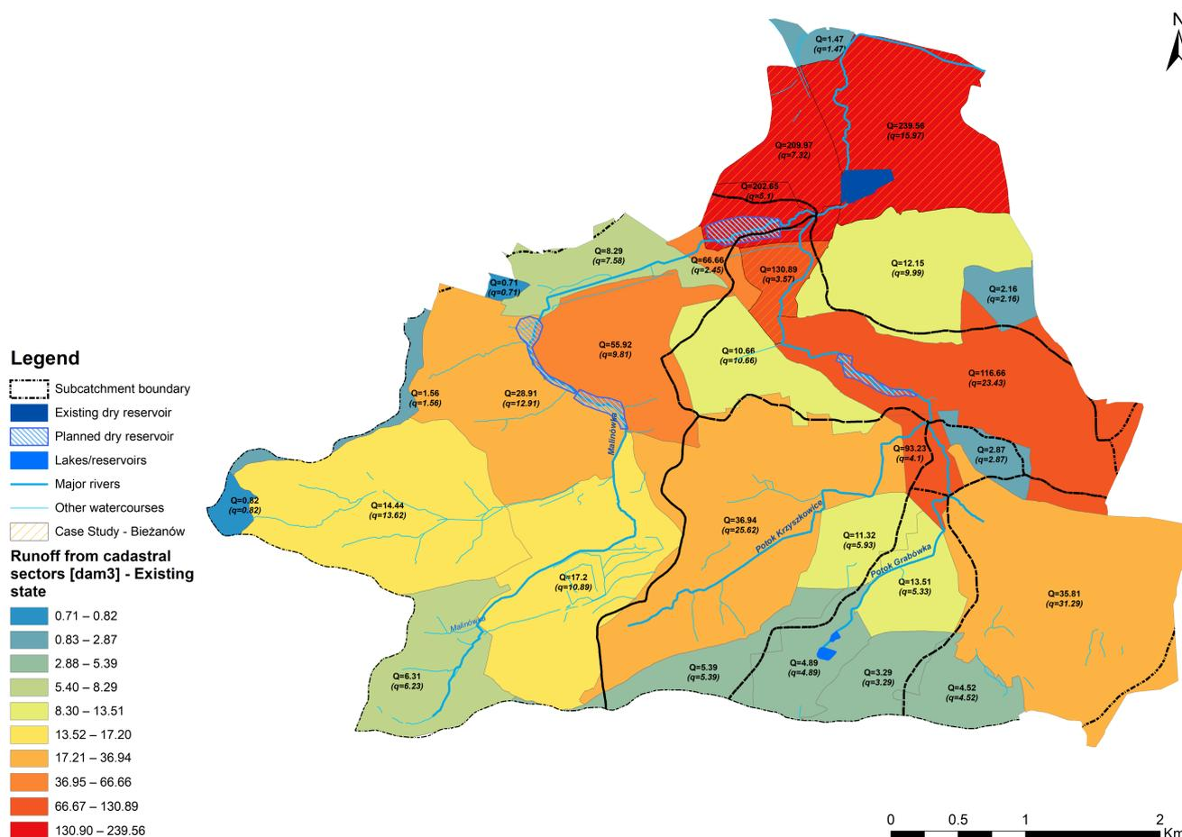
**Figure 8.** Accumulated ( $Q$ ) and specific ( $q$ ) runoff [dam<sup>3</sup>] in each cadastral sector.
