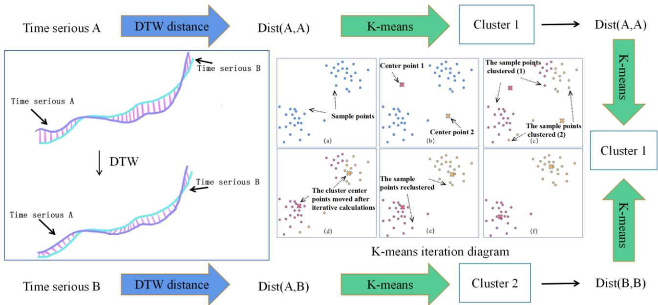
**Figure 3.** The basic steps of the DTW+K-means algorithm.
