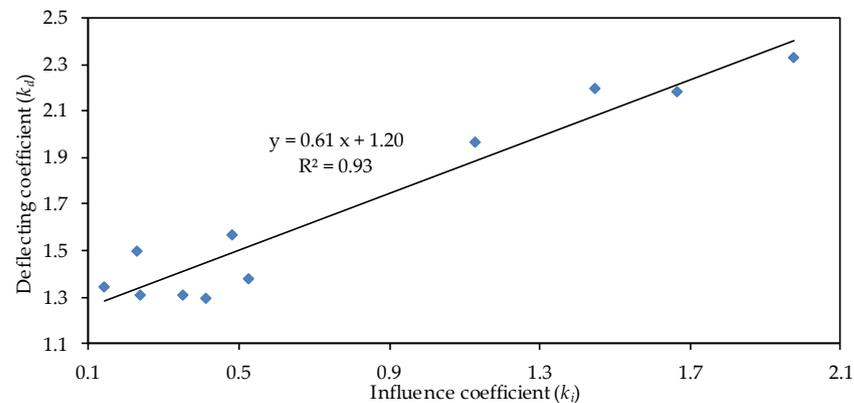
**Figure 9.** Relationship between the influence and deflecting coefficient of the nodes in branching rivers.
