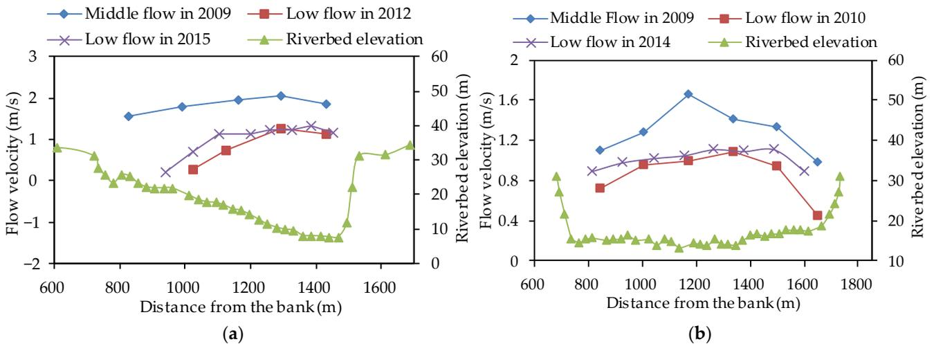
Figure 7. Main flow migration during the middle-flow period: (a) V-shaped section in Tiaoguan reach; (b) U-shaped section in Tiepu reach.
