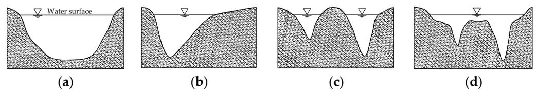
**Figure 4.** Schematic diagram of different cross-sectional shapes: (a) “U” shape; (b) “V” shape; (c) “W” shape with an emersed sand bar; (d) “W” shape with a submarined sand bar.
