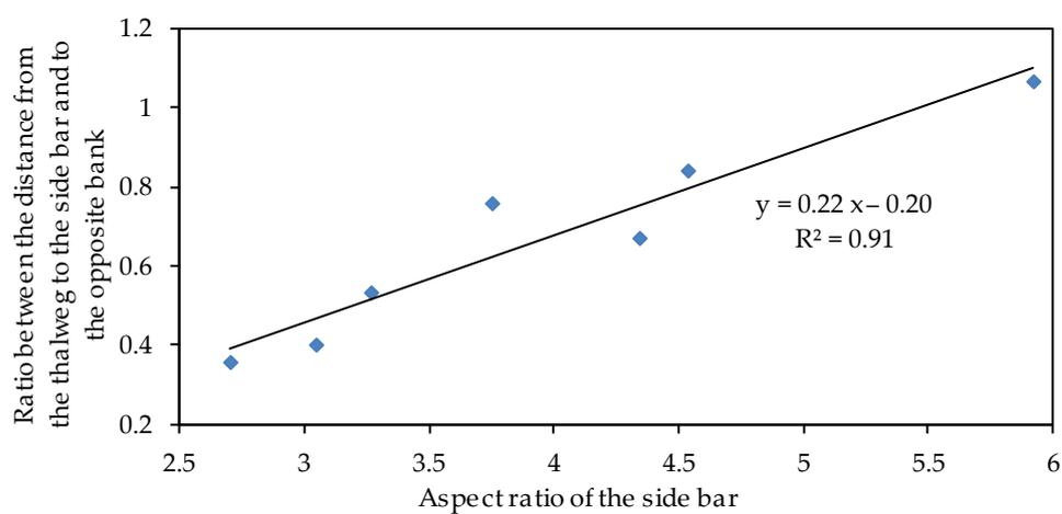
**Figure 11.** Relationship between the relative position of thalweg and the aspect ratio of the side bar.
