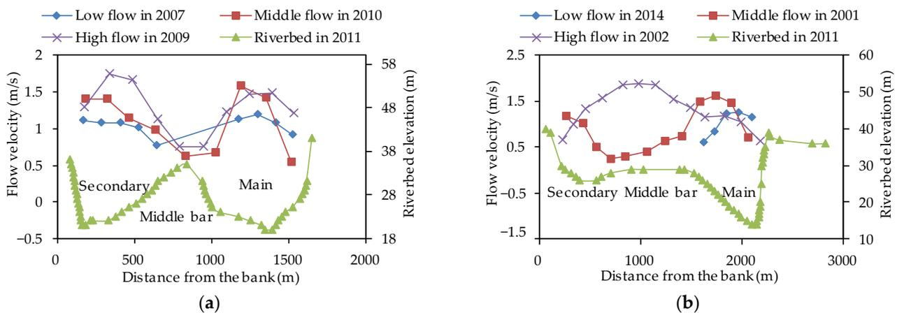
**Figure 8.** Main flow migration during high flow: (a) Taipingkou reach; (b) Majiazui reach.
