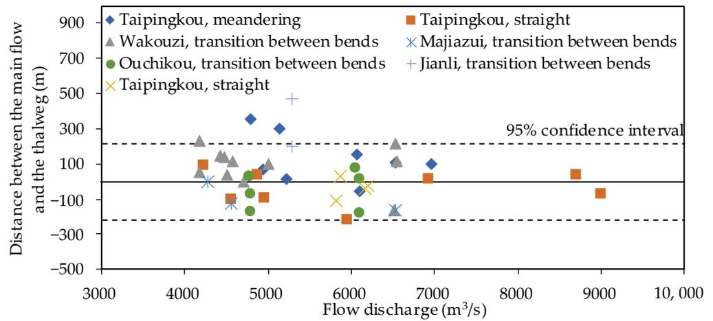
**Figure 3.** Distance between the main flow and the thalweg in Jingjiang reach during the low-flow period.
