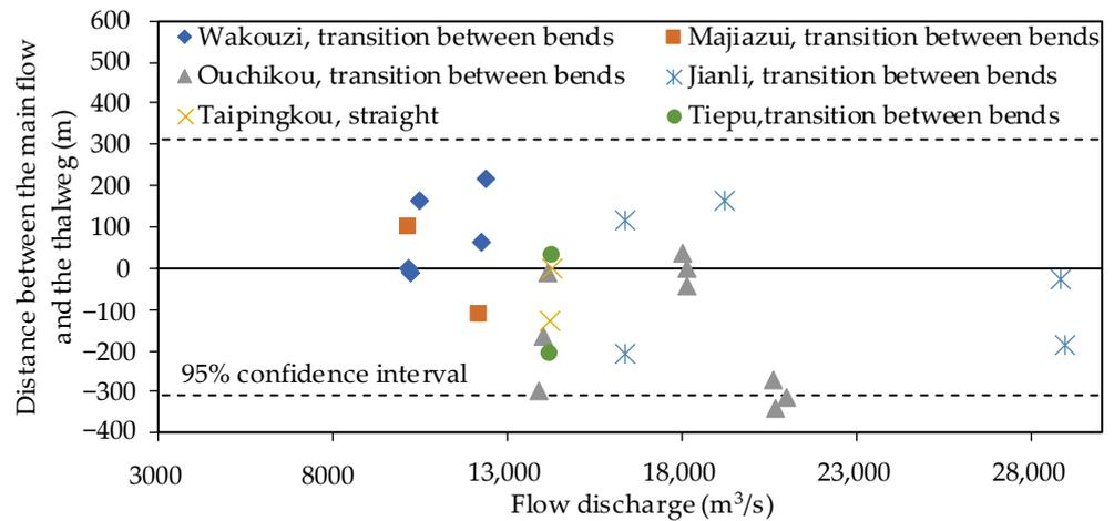
Figure 6. Distance between the main flow and the thalweg for the reach with river width less than 1200 m in Jingjiang reach during the middle-flow period.
