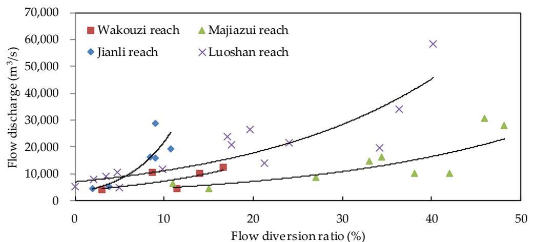
**Figure 13.** Relationship between the flow discharge and diversion of the secondary branch in branching reaches.
