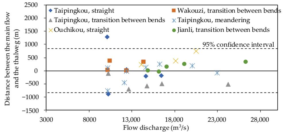
Figure 5. Distance between the main flow and the thalweg for the reach with river width greater than 1200 m in Jingjiang reach during the middle-flow period.
