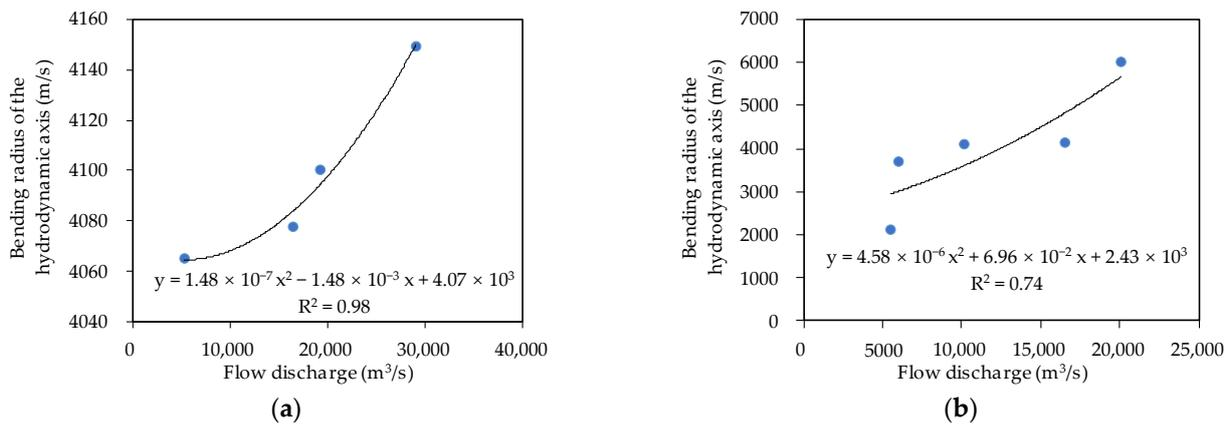
**Figure 12.** Relationship between the bending radius of the hydrodynamic axis and the flow discharge: (a) Jianli reach; (b) Shashi reach.
