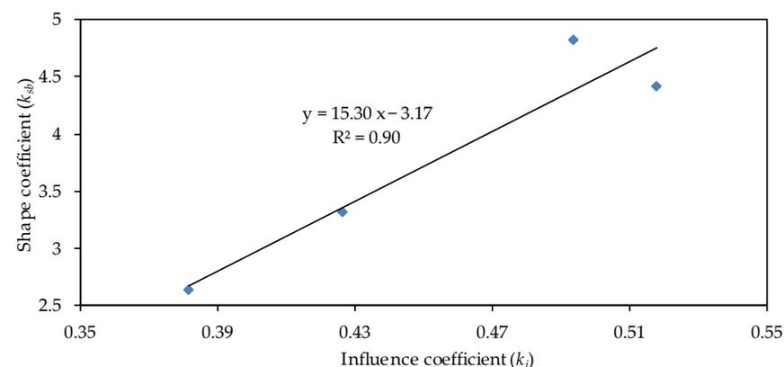
**Figure 10.** Relationship between the influence and shape coefficient in straight rivers with a side bar.
