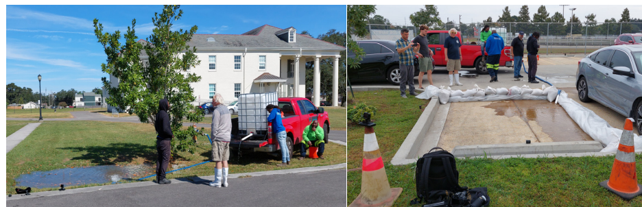
Figure 5. (Left) FSIT at raingarden Milne (test number G14, Table 1). (Right) FSIT at permeable pavement after building a confined space with plastic and sandbags.
