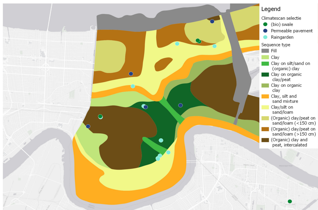
Figure 3. Lithological sequence type map constructed based on borehole information. Source Digital Elevation Model: Deltares (2022).
