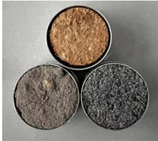
**Figure 1.** Three different soil porous media that are uniformly placed in a circular bowl. The soil samples were exposed to an air-dried environment and used to measure total soil porosity.
