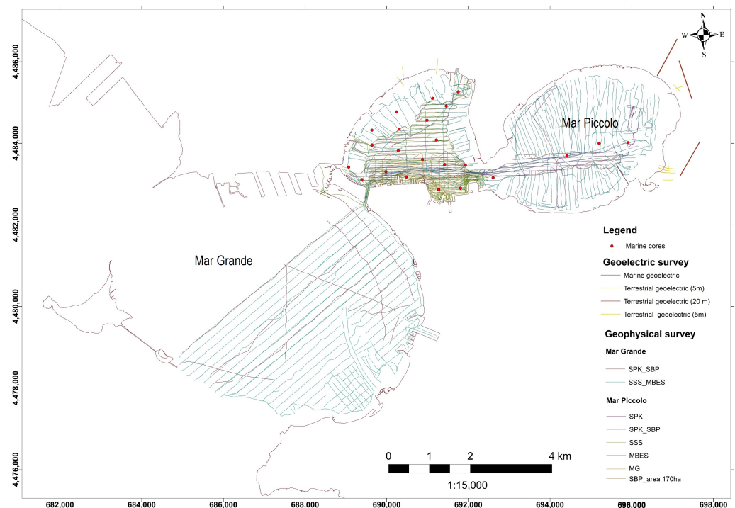
Figure 7. Navigation lines followed for the geophysical and geoelectric surveys carried out in the frame of the activities funded by the Special Commissioner. The positions of the 24 sediment cores carried out in the Mar Piccolo are also indicated.
