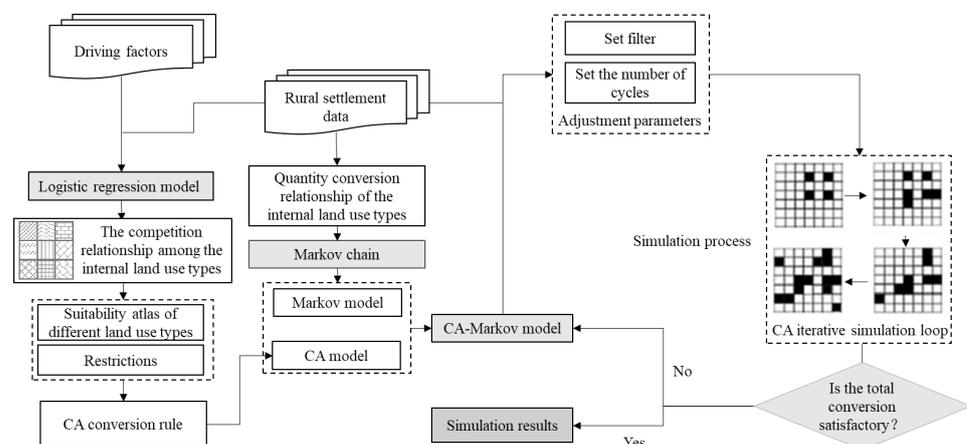
Figure 3. CA–Markov model simulation process.
