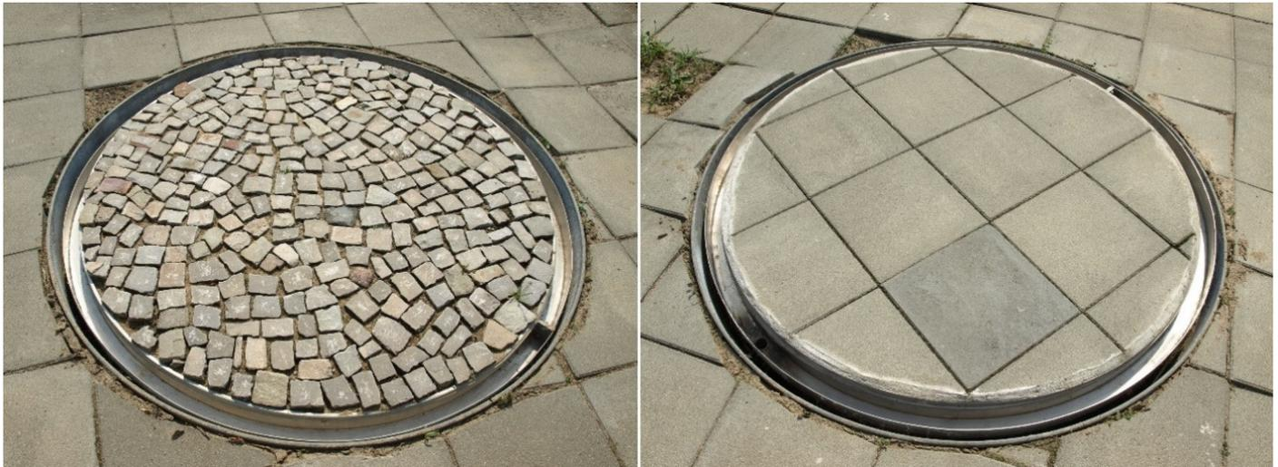
**Figure 1.** Lysimeter surfaces: (left), cobble-stones; (right), concrete slabs. Reprinted with permission from Timm [22].
