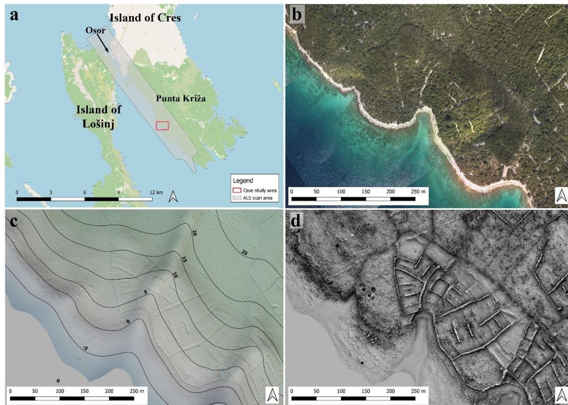
**Figure 2.** (a) Map of the total area of ALS data capture and the case study area (red box). (b) Ortho-photograph of the case study area produced simultaneously with ALS data acquisition (March 2012). (c) Contour lines at 5 m intervals calculated based on low pass filtered digital feature model (DFM;  $r = 20$  m). The zero-contour marks the coastline. (d) Filtered DFM (visualization: cVAT).
