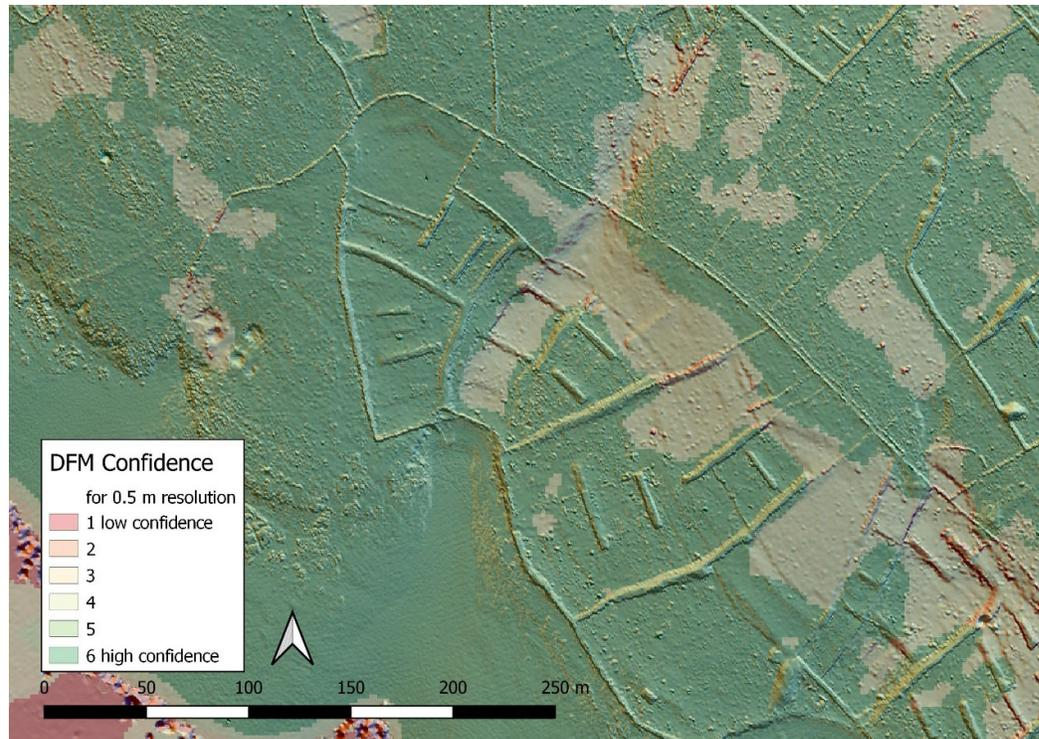
**Figure 7.** DFM confidence map showing the suitability of the ground point distribution for a DFM grid size of 0.5 m after classification using the “stone\_wall” setting. Almost the entire area shows classes ranging from 4 to 6, which is adequate for interpolation using a 0.5 m grid.
