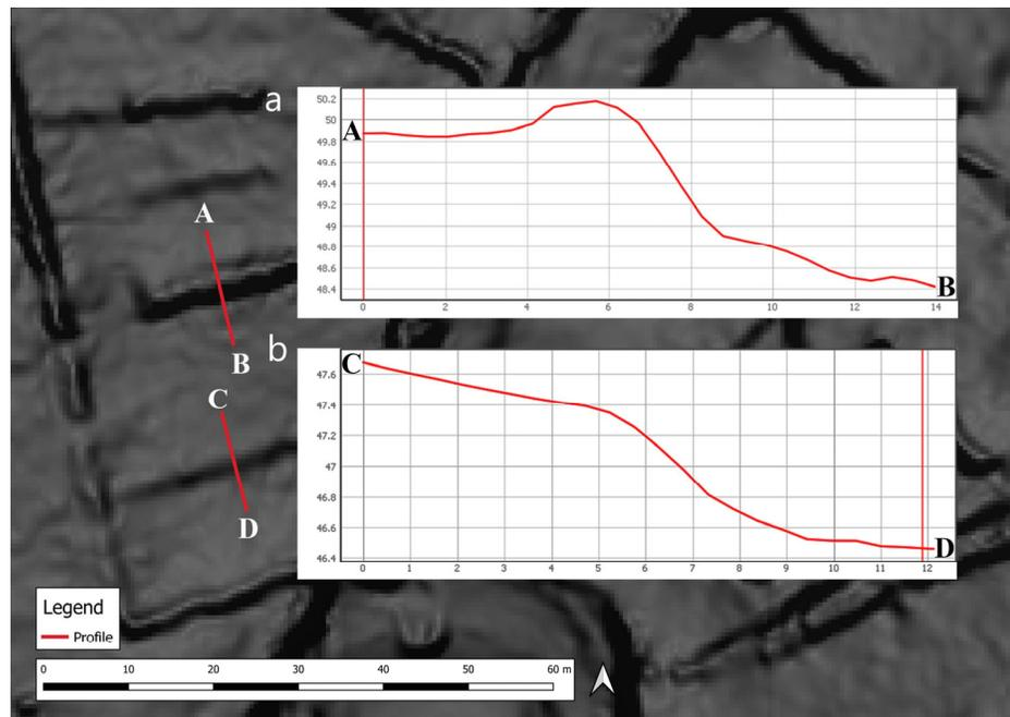
**Figure 24.** Screenshots of a QGIS session using the profile tool. (a) Surface profiles help to distinguish terrace slopes (b) from slopes that are overlain by a stone deposit (visualization: slope).
