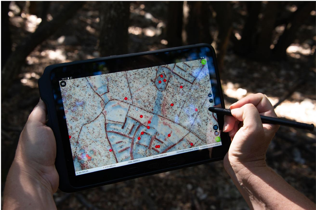
**Figure 9.** The tablet device in the field. QField was used to view and edit GIS layers in the field, with the current GPS position visible on the screen (the small white dot in the centre of the tablet). (Photo: M. Doneus, 1 September 2021).
