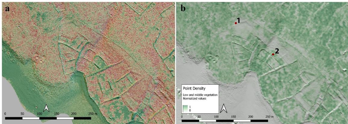
**Figure 6.** (a) Map showing the density of ground points after ground point filtering using the “stone wall” setting. Red colours indicate densely vegetated areas with low penetration rates. (b) A point density map of low and medium height vegetation (0–1 m) provides a good estimate of accessibility for ground observation. The red dots show the locations of ground photographs. Nr. 1: Figure 18, Nr. 2: Figure 16E.
