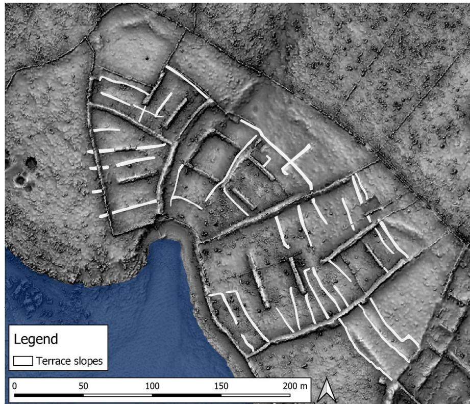
**Figure 25.** Interpretative mapping of terrace slopes (visualization: combination of slope, hillshade, and Negative Openness ( $r = 10$ )).
