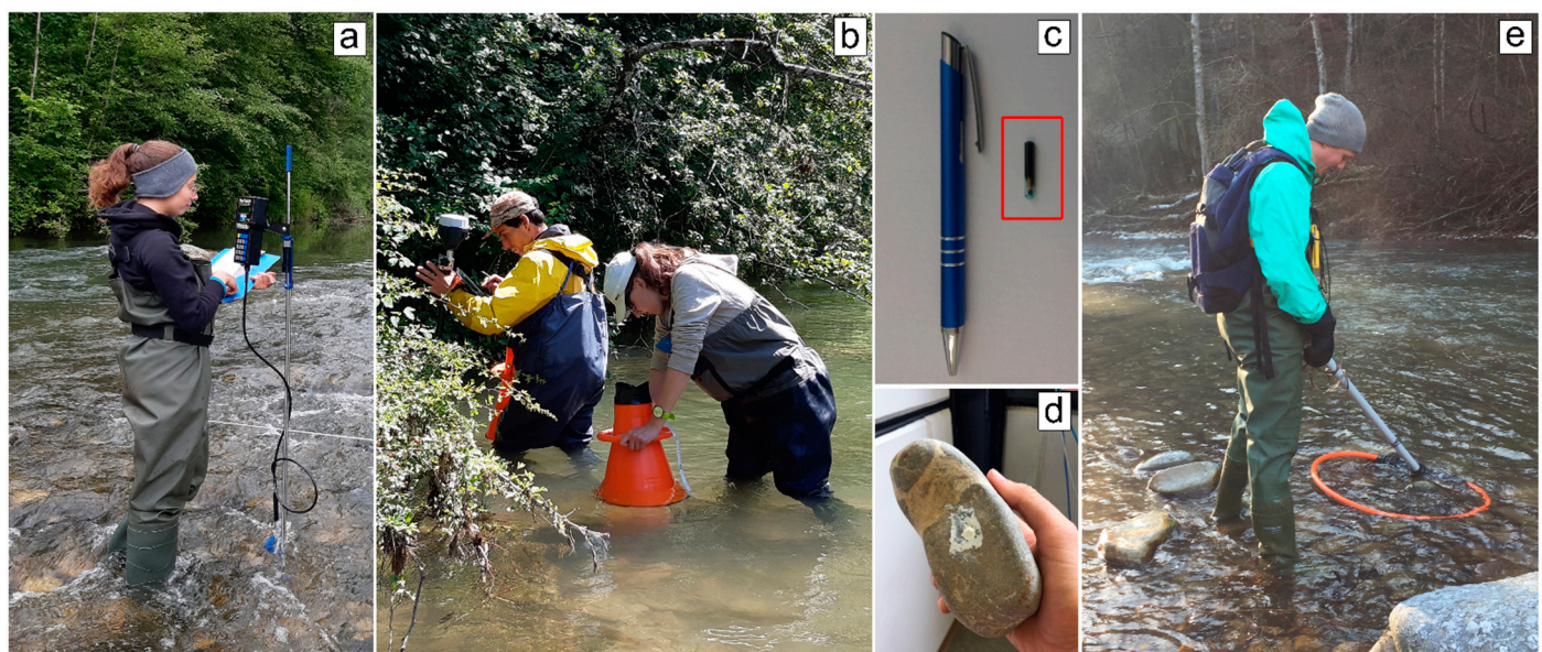
Figure 4. Assessment of the eco-morphological effectiveness of a sediment augmentation measure: (a) recording flow velocities and water depth along fixed cross-sections, for the calculation of the HMID abiotic indicator; (b) mapping substrate quality for the calculation of the IRS [113] abiotic indicator; (c) RFID-pit sensor; (d) a pebble with an RFID-pit sensor inside; (e) post-flood bedload tracing, searching for the RFID-pit sensor pebble with a mobile antenna.
